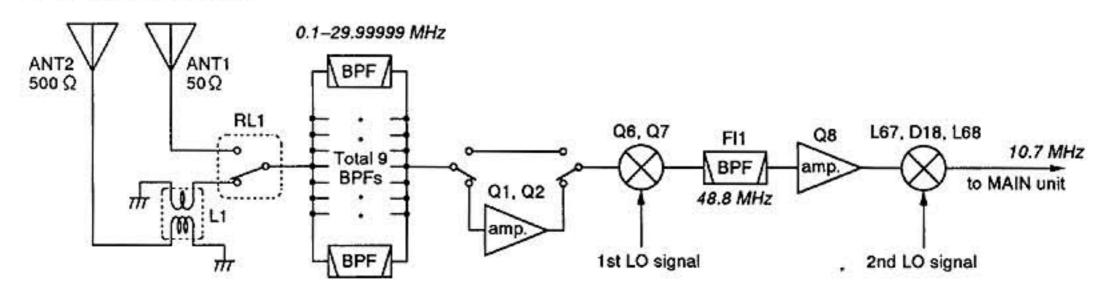
Then the RF signals from the switching diode (D17) are applied to the 1st mixer circuit.
