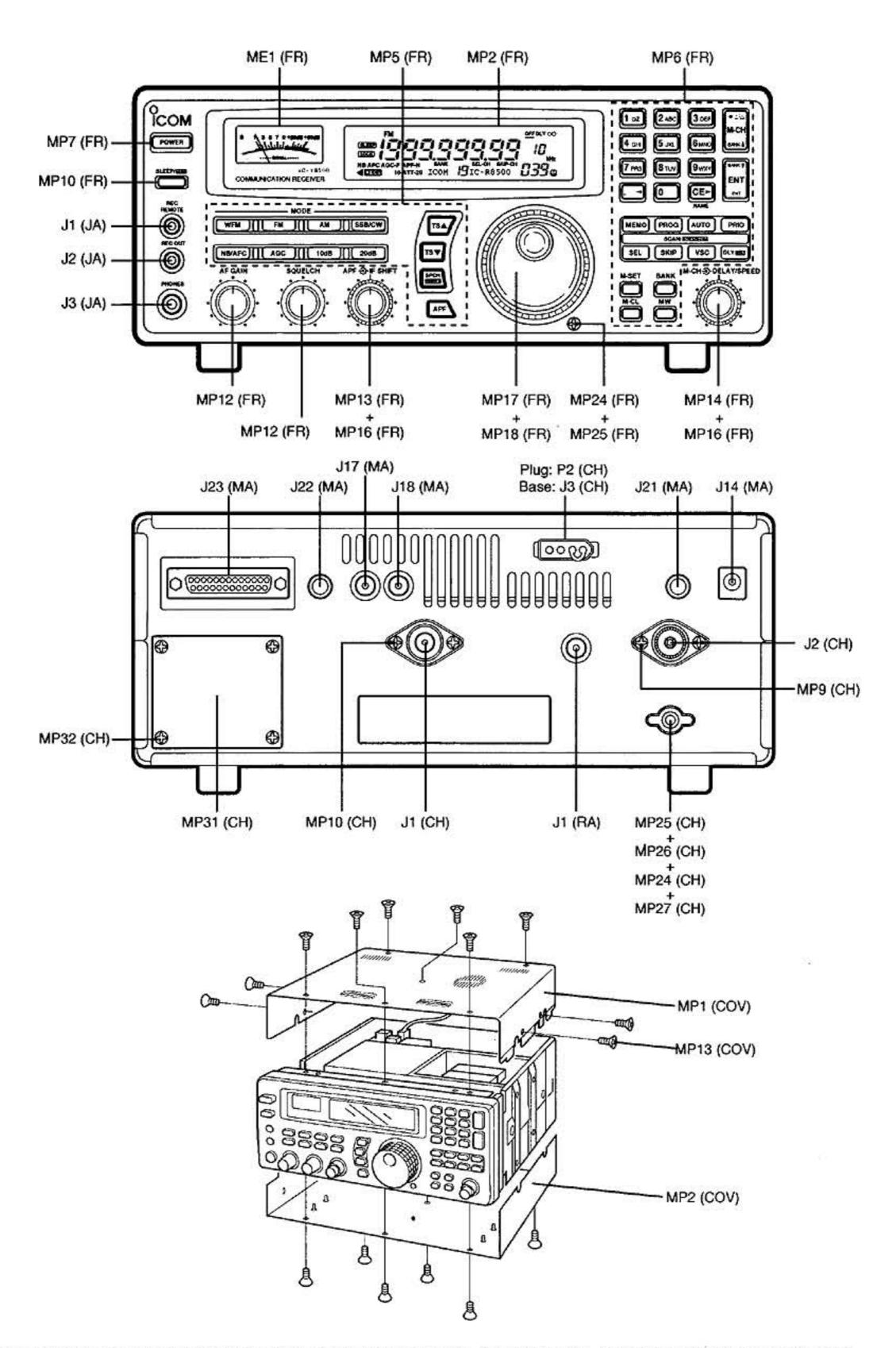
Unit abbreviations (CH): CHASSIS PARTS (FR): FRONT PARTS (D): DISP UNIT (RA): RF-A UNIT (MA): MAIN UNIT (COV): COVER PARTS (JA): JACK BOARD (VA): VR-A BOARD (VB): VR-B BOARD
