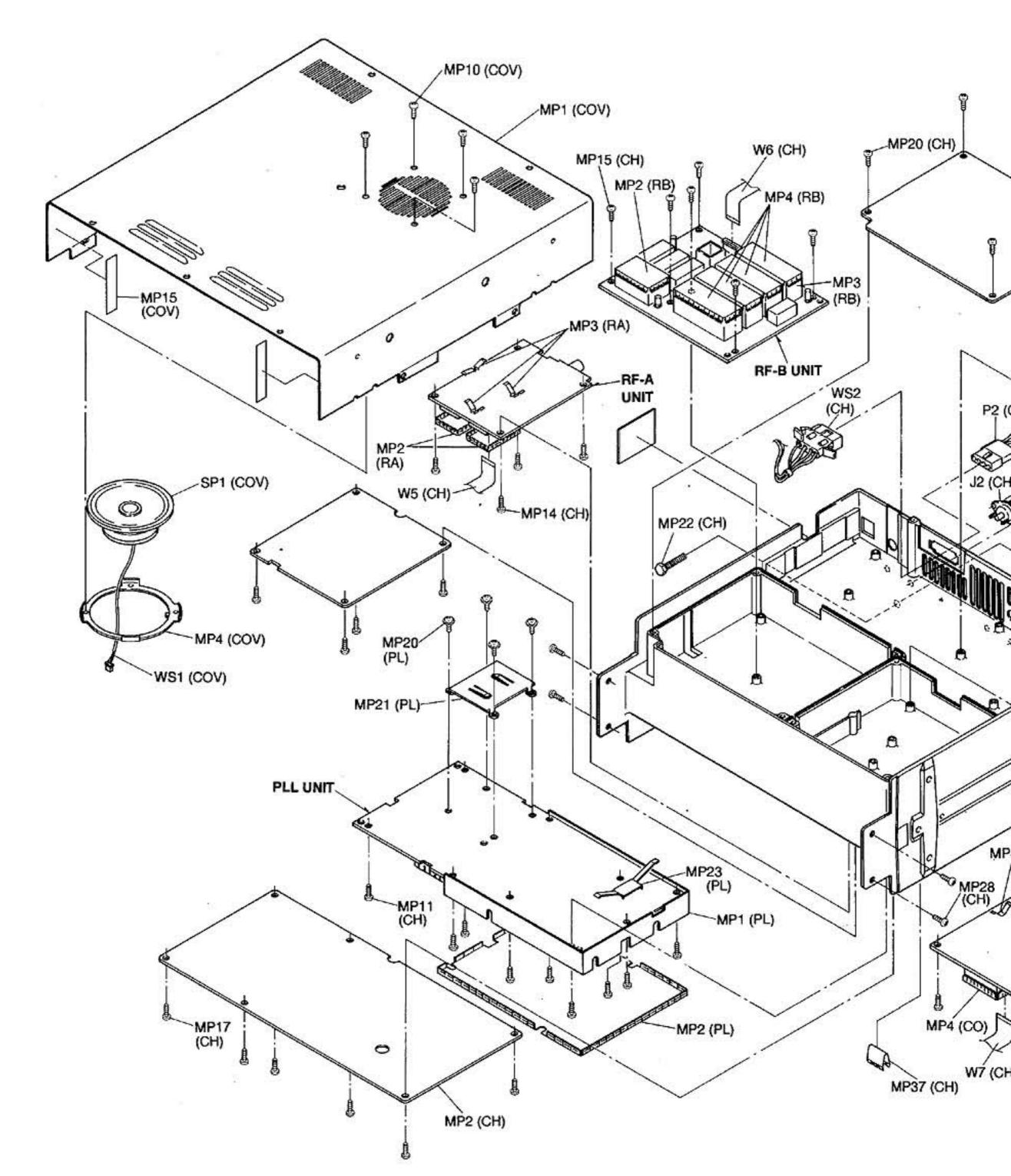
Unit abbreviations (CH): CHASSIS PARTS (MA): MAIN UNIT (PL): PLL UNIT (RA): RF-A UNIT (RB): FR-B UNIT (CO): CONV UNIT (MI): MIX UNIT (COV): COVER PARTS
